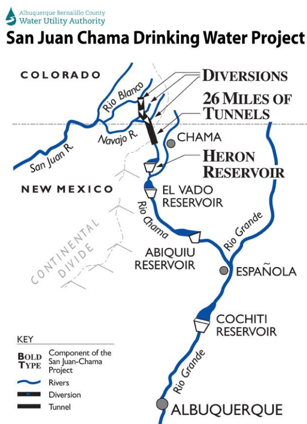
Figure 1 Interbasin transfer of Colorado River water via the San Juan-Chama Project. ABCWUA.
